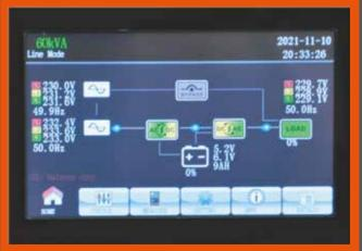
With the easy to read multifunctional LCD display everything is under control. Thanks to new advanced LCD screen, input-output values and alarms can be easily monitored.
